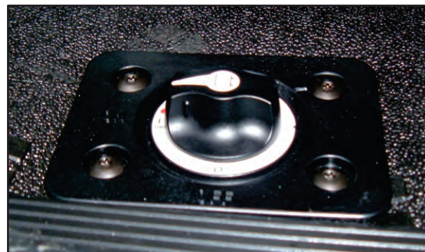
293-058/-060/-061 Positive Disconnect Switch
